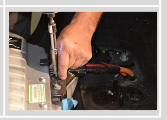
Remove the two 10mm bolts securing the HV leads to the battery, and the one 10mm grounding bolt.
