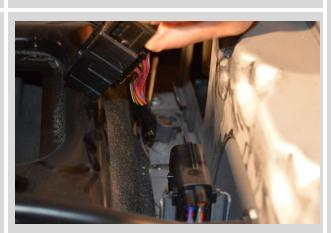
Disconnect black wire harness by pulling upwards and folding back.
