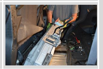
Follow these same steps in reverse to install the replacement battery from Best Hybrid Batteries
