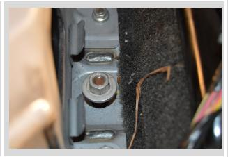
Remove two 18mm nuts on the front side of the battery.
